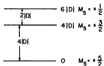
Figure 2. Negative axial zero field splitting for high spin Fe(III)
